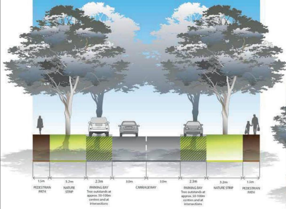
Figure 12: Typical Local Access Street Level 2 Cross Section
