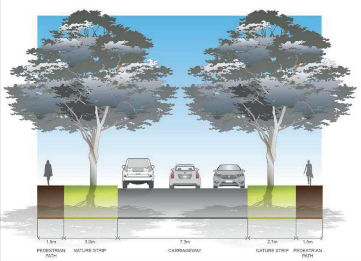
Figure 13: Typical Local Access Street Level 1 Cross Section
