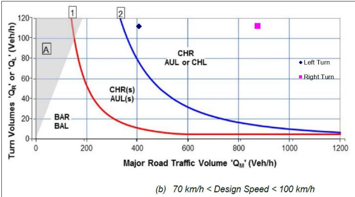
Figure 17: Geelong-Ballan Road Site Access Connection - Turning Lane Warrants (PM Peak Hour)
