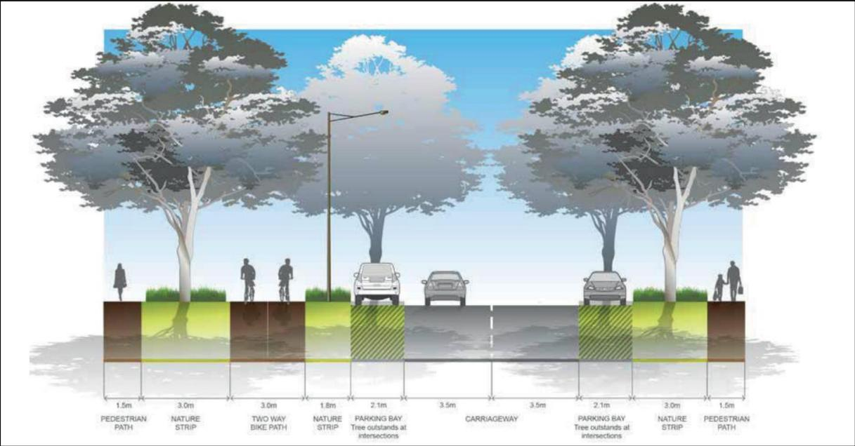
Figure 11: Typical Connector Street Cross Section
