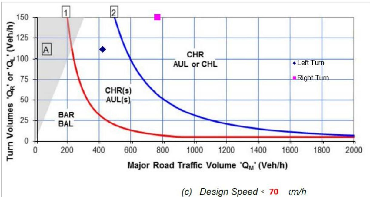
Figure 18: Old Melbourne Road Site Access Connection - Turning Lane Warrants (PM Peak Hour)
