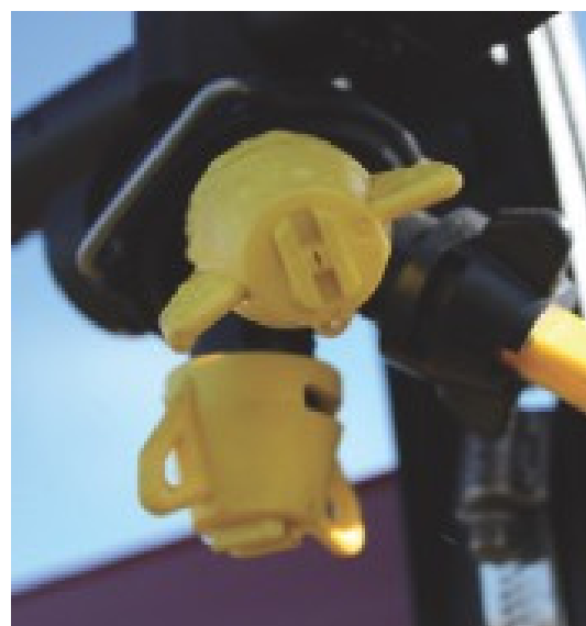
Triple nozzle system on a boom
