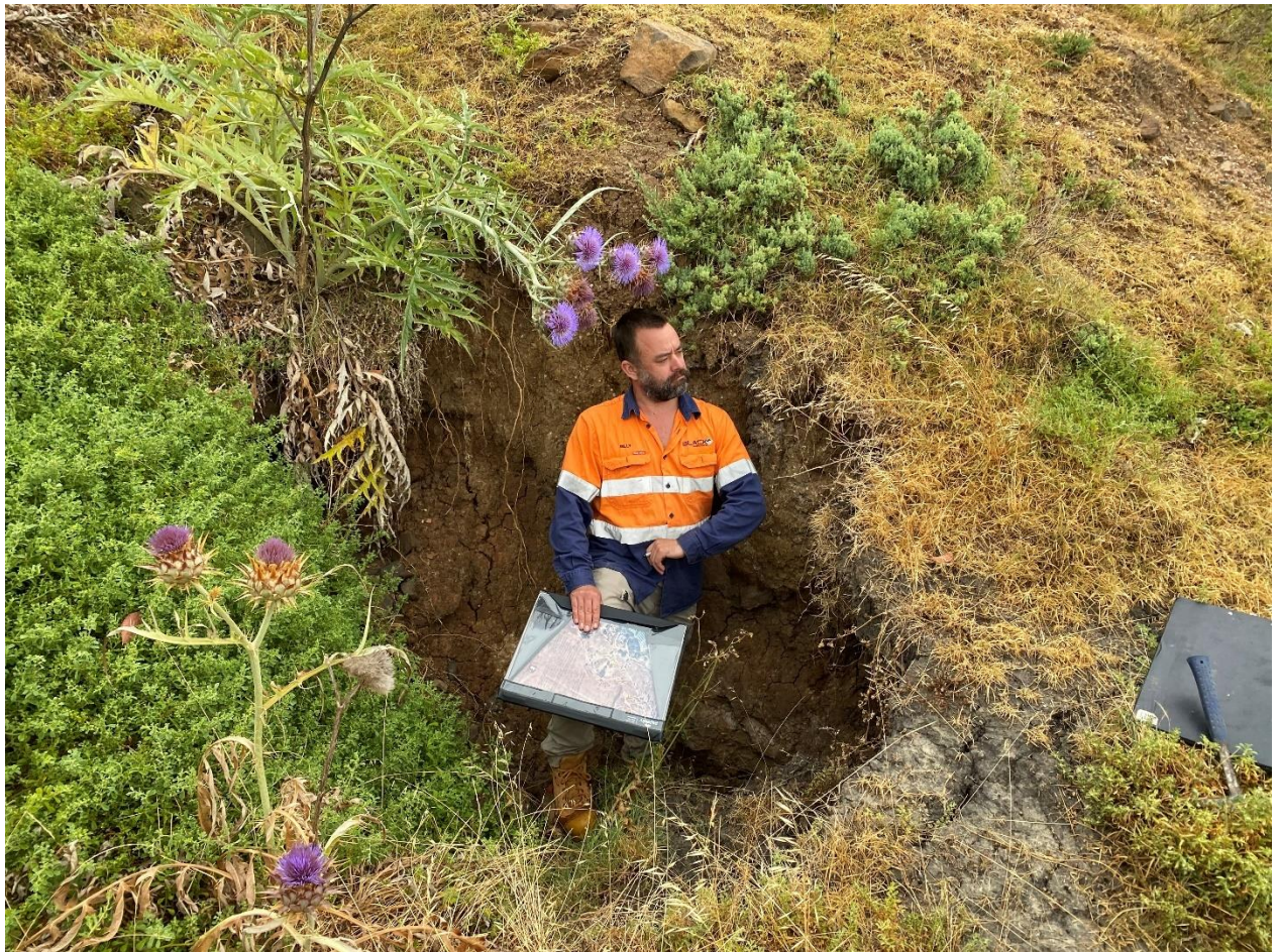
Image 24 – Large solution feature above filled quarry/sand pit, located north of subject site in DOTP road reserve.
