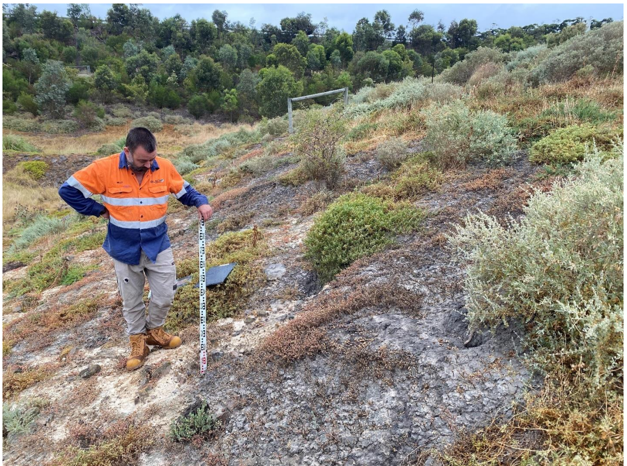
Image 25 – 1.9 m deep solution hole towards base of filled quarry/sand pit in DOTP road reserve.
