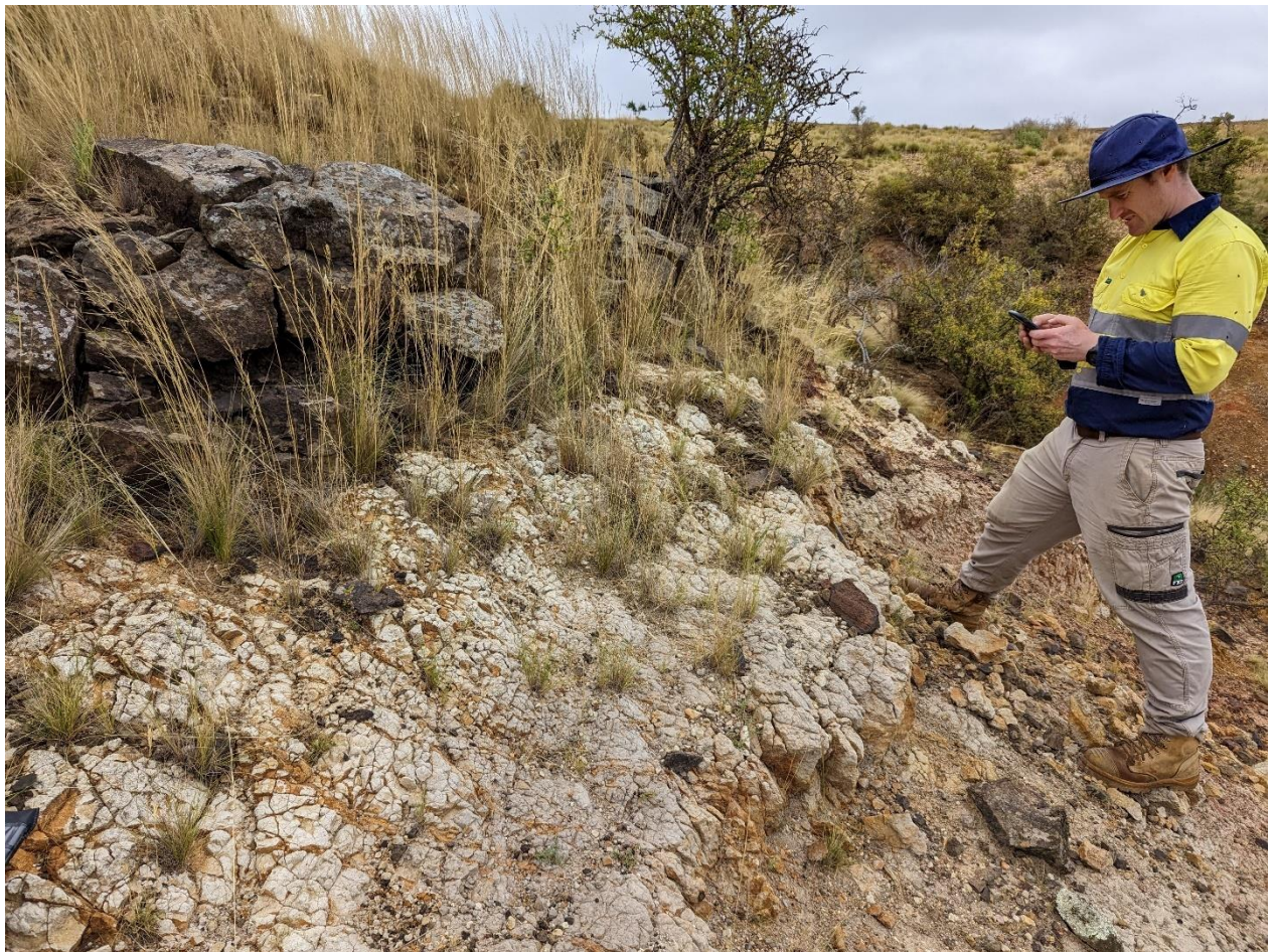
Image 23 – Clear geological contact between basalt and Werribee Formation.
