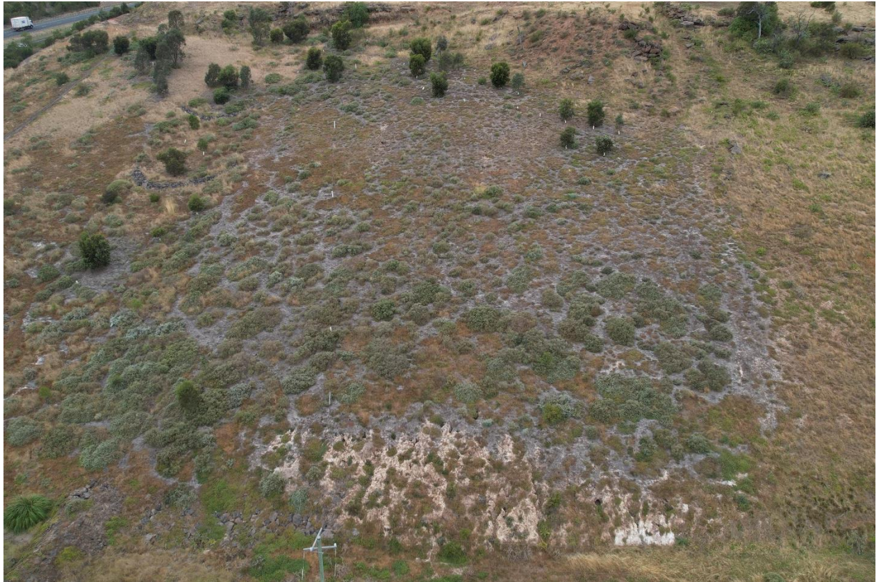
Image 26 – Aerial view of failing fill (grey and white material), located north west of subject site in DOTP road reserve.
