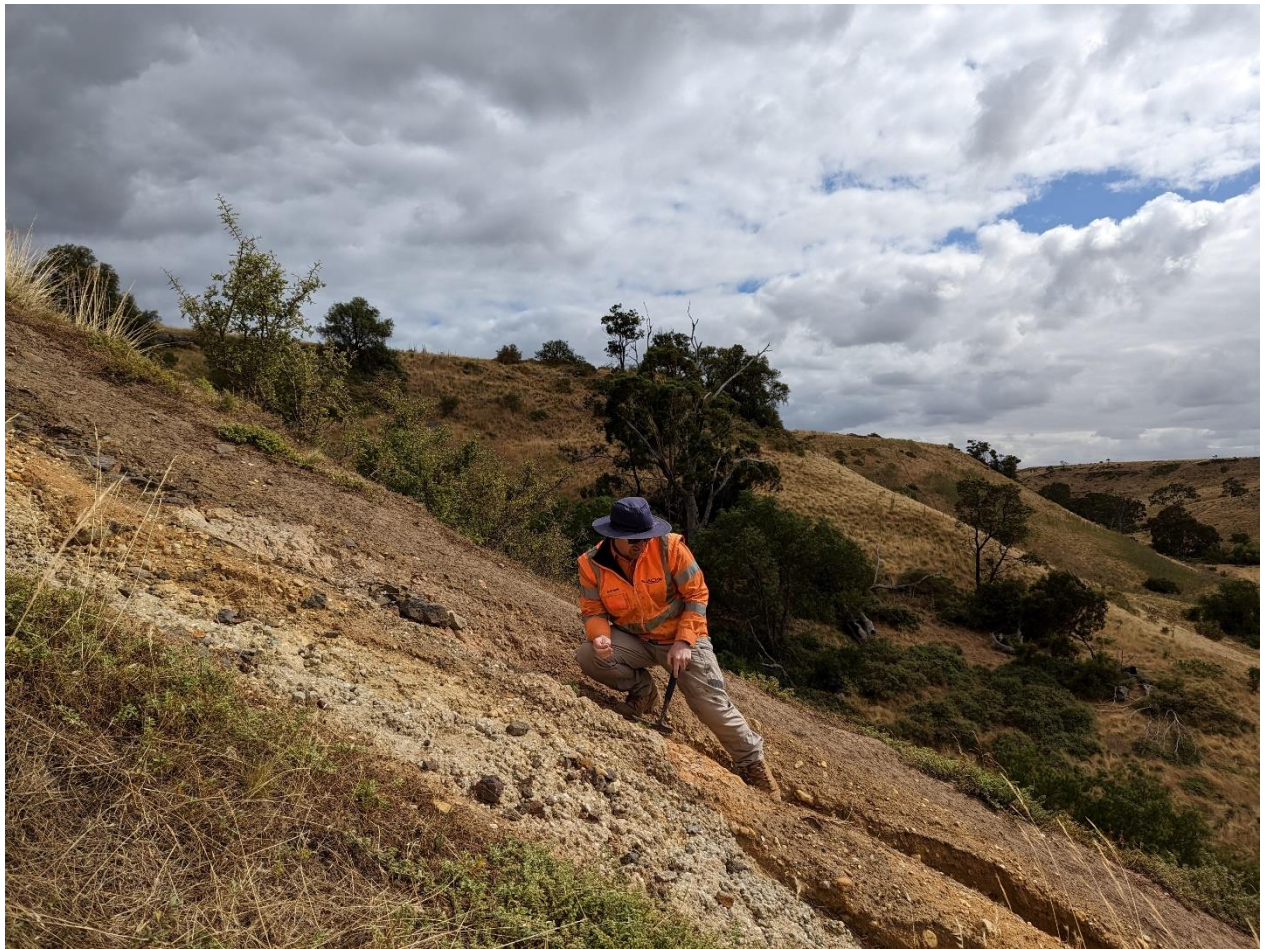
Image 11 – Geological contact between basalt and underlying Riddell Sandstone. Steepness of track is evident.
