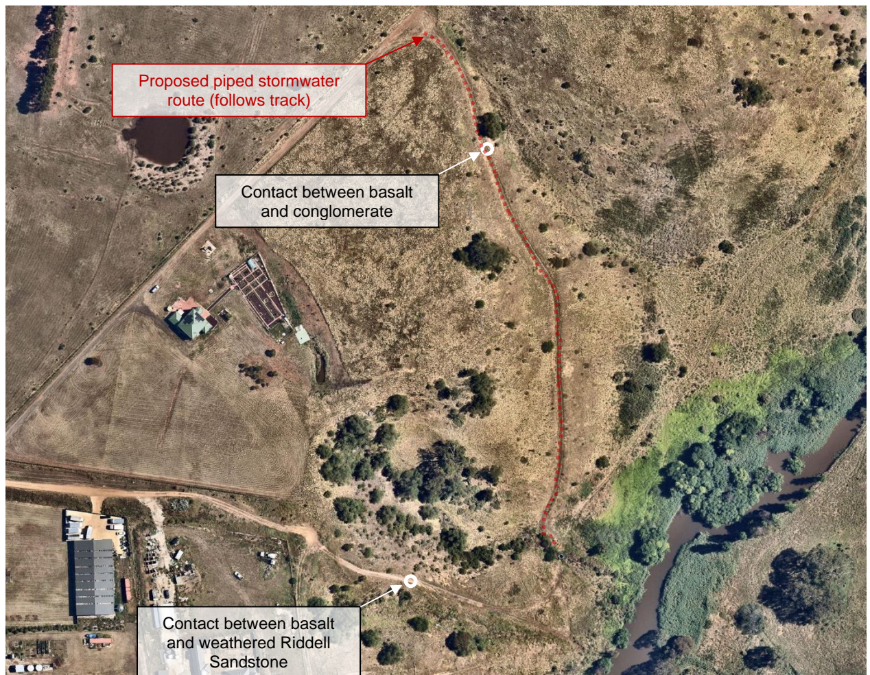
Image 9 – Marked up Nearmap image with geological contacts and proposed pipeline route.
