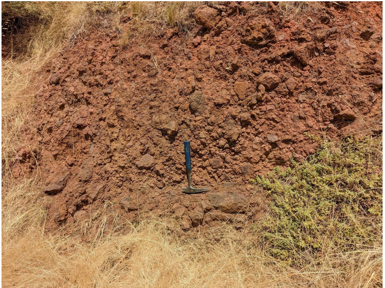
Image 13 – Base of basalt / potential contact with colluvium above less steep track.
