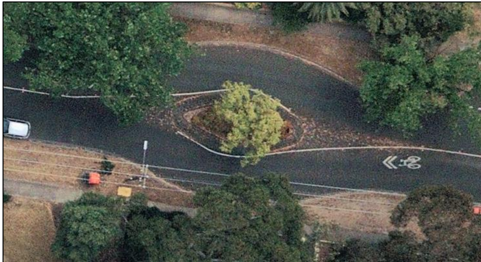
Figure 4 Example of centre blister island (from Nearmap aerial photography)
