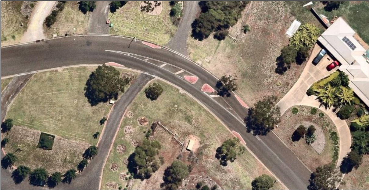
Figure 13 Existing LATM treatment on Manning Boulevard
